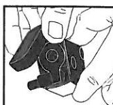
**STEP 1. Unplug unit. Remove pump intake top cover.**
